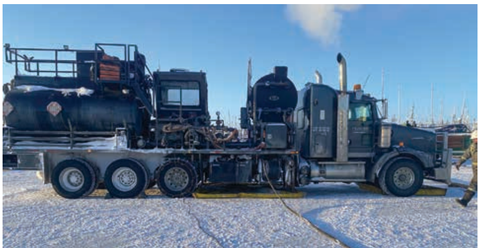
Hot oiler and methanol injector near Colville Lake, March 2026. (Credit: OROGO)
